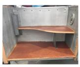
Progress on single-deck Daimler CVD6 has been good in the last month with the fitting of the rebuilt entrance steps. We will need to rebuild the entrance doors next and find a suitable bottom pivot bearing to install the doors. Rebuilding of the cab front has commenced and completion of the offside wing which forms the cab floor is imminent. The emergency exit door and the cab door are under way and just waiting for parts at present.
