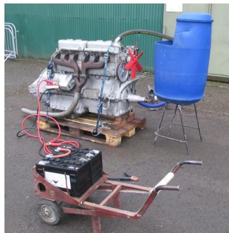
Pic of 14's engine set up to test run with "temporary radiator".
